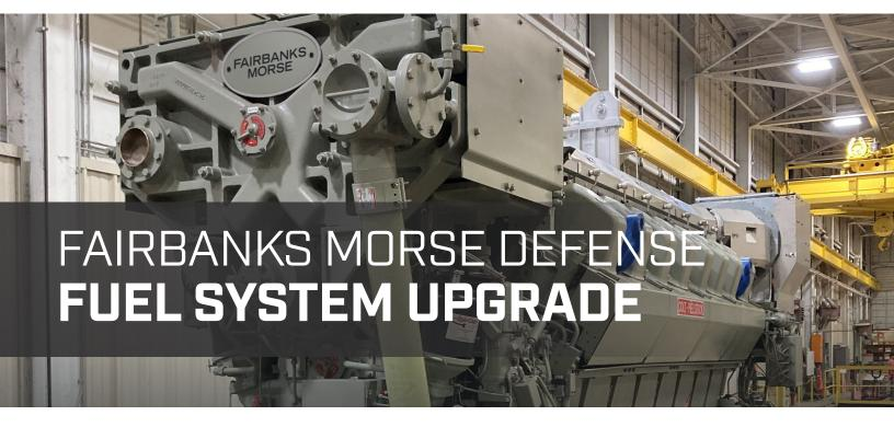
The FM PA6B Fuel System Upgrade is a comprehensive fuel system upgrade optimizing the fuel delivery and efficiency of the PA6B engine. The upgrade includes a conversion to electronic fuel injection and upgrading the existing injection nozzles using modern manufacturing techniques and improved materials to increase the nozzle hydraulic efficiency and fuel atomization.
