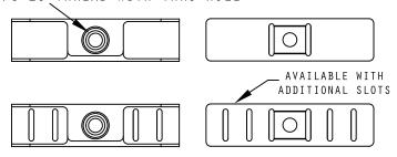
MAX LOAD: 2 TIER OFF BULKHEAD, 3 TIER OFF OVERHEAD
