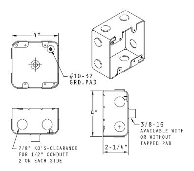
DRAWN 4X4 SQUARE UTILITY BOXES ARE AVAILABLE WITH WELDED STUDS FOR EASY MOUNTING TO THE SHIP'S BULKHEAD. STEEL BOXES ARE ELECTROGALVANIZED.
