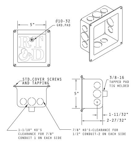
DRAWN STEEL 5X5 OVERSIZE SQUARE UTILITY BOXES HAVE WELDED STUDS FOR EASY MOUNTING TO THE SHIP'S BULKHEAD. BOXES ARE ELECTROGAL-VANIZED.
