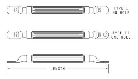
CATALOG NUMBERING SYSTEM MIL-STD-1310 REV E TYPE 1 AND TYPE 2 BONDING STRAP
