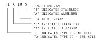
BOND STRAPS ARE MADE WITH TRXF84 CABLE ADDITIONAL LENGTHS AVAILABLE
